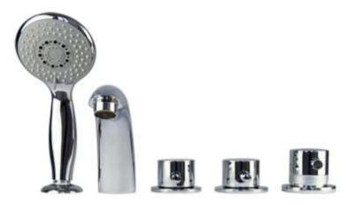
Ella Acrylic Walk In Bathtubs have the option to include an Ella Standard 5 Piece Faucet Set that comes with a Deck Mounted Thermostatic Control Valve (TCV), which is an anti-scald feature that keeps the water at a consistent temperature and prevents water from suddenly shifting to unsafe temperature levels.
