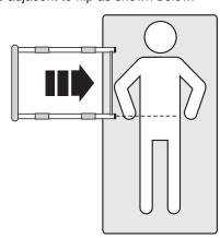
**A2.** Align rail with edge of bed. Align female side of the buckle close to edge of bed (NOTE: Length (\*L) of strap from knot to edge of bed depends on size of bed). Tie a knot around the rail leg as shown in the inset (1) of **Figure 1**. Pull strap across and tie a knot around the other rail leg (2). Pull strap around metal bed frame (3). Put the mattress back on the box spring and pull slack to tighten strap (4).
